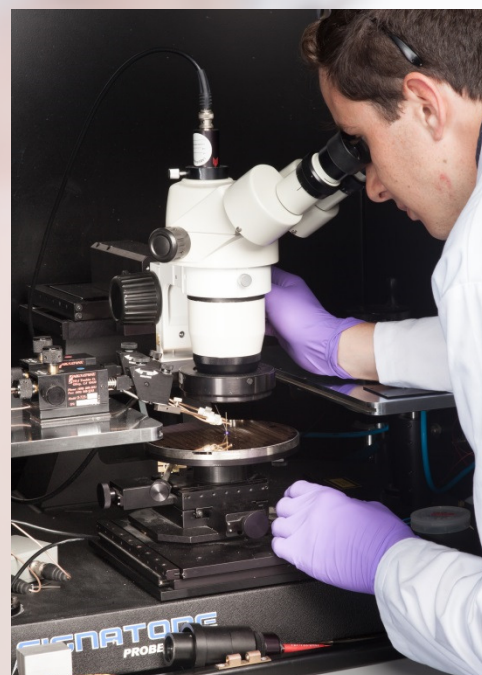
John working on our LED probe station, testing the device performance of our samples.
