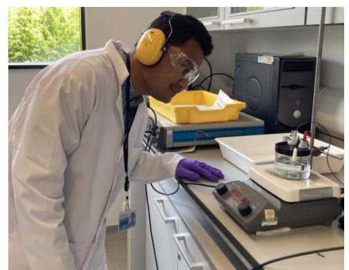
Galih doing an electrochemical etching experiment to synthesize porous GaN.
